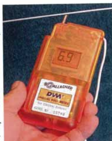
Fig. 3. A digital voltmeter is an essential tool for electric fences.
